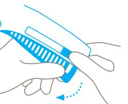
Swing the lever completely **out of the handle**, and flip open the blade cover.
