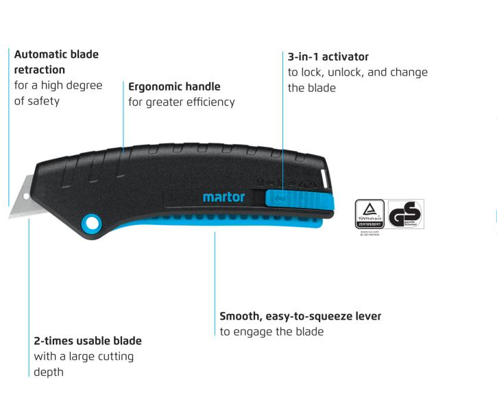
To **engage the blade**, unlock the cutter and squeeze the lever. Now you can cut.
