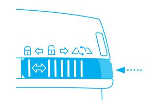
Use the 3-in-1 activator to lock your cutting tool after cutting.
