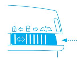
Swing the lever back into the handle and set the 3-in-1 activator to either lock or unlock.
